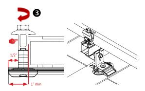
**INSTALL END MODULE:** Position first module onto rails and engage module frame with end clamps. Hold clamp in place against module while tightening bolt.
