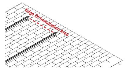
**ALIGN RAILS:** Align one pair of rail ends to the edge of the installation area. The opposite pair of rail ends will overhang installation area. Do not trim them off until the installation is complete. Install the first module at the aligned end. If the rails are parallel to the rafters, the aligned end of the rails should face the lower edge of the roof. Securely tighten all hardware after alignment is complete.
