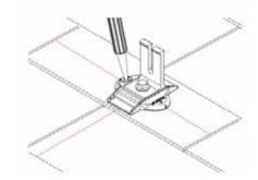
**SEAL:** Insert tip of UNIRAC provided sealant into port. Inject until sealant exits vent. Follow sealant manufacturer's instructions and cold weather application guidelines, if applicable
