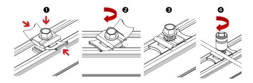
**SYSTEM GROUNDING WITH MLPE & LUG CLAMP:** Insert the rail nut profile in the opening by lifting the flaps of the plastic clip. Rotate the clamp 90 deg and release the flaps to get flush with rail. Ensure that the rail nut is engaged in the rail profile. Align the ground wire in the depression of the washer. Tighten bolt.
