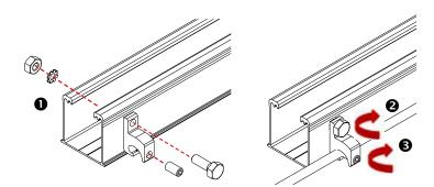
**ALTERNATE SYSTEM GROUNDING WITH ILSCO LAY-IN LUG - UNIRAC P/N 008009P:** Alternate Grounding Lug. Drill hole in rail 7/32" in diameter, deburr hole and bolt thru one wall of rail.
