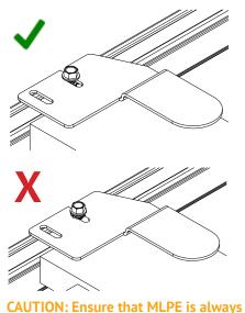
CAUTION: Ensure that MLPE is always installed on the top of lock-tooth washer.
