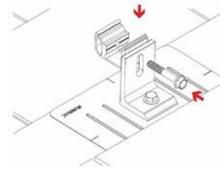
FIX RAIL CLAMP ONTO L-FOOT: Remove bolt from rail clamp. Place bolt through slot in L-foot and though hole in Rail Clamp. Partially thread holt into rail clamp, leaving the bolt loose to accept the rail.
