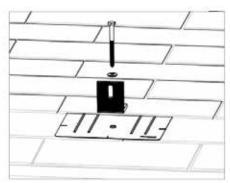
INSTALL L-FOOT: Fasten L-foot and Flashing into place by passing the included lag bolt and pre-installed stainless steel-backed EPDM washer through the L-foot EPDM grommet, and the hole in the flashing, into the pilot hole in the roof rafter. Drive the lag bolt down until the L-foot is held firmly in place. The EPDM washer should compress and expand slightly beyond the outside edge of the steel washer when the proper torque is applied.
