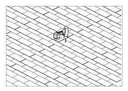
**DRILL PILOT HOLES:** Drill a 7/32" pilot hole at each roof attachment. Clean roof surface of dirt, debris, snow, and ice. Fill each pilot hole with sealant.
