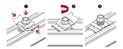
**INSTALL MLPE & LUG CLAMP:** Insert the rail nut in the rail by pinching the flaps of the plastic clip with thumb and middle finger, while pressing bolt head down with pointer finger. Rotate the clamp 90 deg in clockwise or anticlockwise in the rail and release the flaps when aligned with rail. Ensure that the rail nut is engaged in the rail profile.
