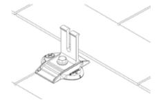
CAUTION: WHEN INSTALLING THE STRONGHOLD ATTACHMENT OVER VERTICAL JOINTS, FILL GAP/JOINT WITH SEALANT BETWEEN MOUNT AND UPSLOPE EDGE OF SHINGLE COURSE.
