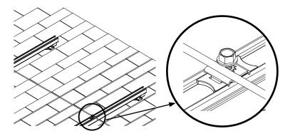
**SYSTEM GROUNDING:** Rails can be bonded using an NXT Horizon MLPE & Lug Clamp, GROUND WEEBLUG #1 or ILSCO LAY IN LUG (GBL4DBT). At least one rail per row of modules in an array must be bonded to electrical ground. Each additional row of modules must be grounded with at least one rail lug per row or with a row-to-row bonding devise listed here.
